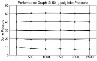
Regulated Pressure @ Variable Flow Rates In CC/Min
